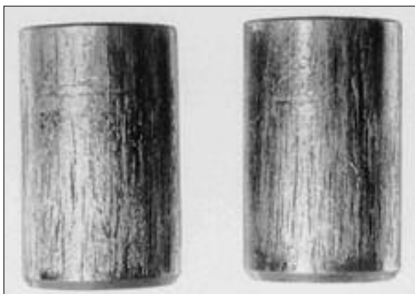
Contaminated hydraulic oil scored these hydraulic pump pistons
